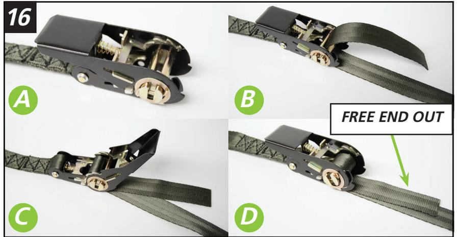
**IMPORTANT: DO NOT** over-tighten these straps to where it starts to pull the foot platform down the tree. **See figure 17.**
