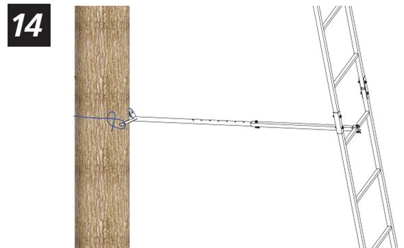
11. Take the two (2) straps that are hanging freely down, walk behind the tree so that the straps form an "X" in the straps as shown in **figure 15**. Pull the straps around to the bottom ladder section and secure the straps to the previously installed ratchet straps below the third ladder rung. **See figure 16, A - D** for proper threading of the ratchet strap. Ensure that the free end in **figure 16, step D** is facing out.
