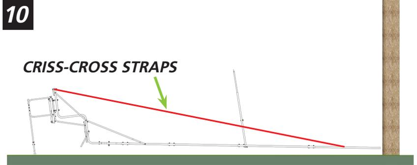
8. With all the straps secured to the stand, you are now ready to raise the ladder stand with three able adults. Starting at the platform area, one person needs to be on each side of the ladder section and one person in the middle. CAREFULLY raise the ladder stand up until the v-bar teeth come in contact with the tree. See figure 11. Pull the end of the ladder sections out away from the tree until the foot platform is level. See figure 12.
